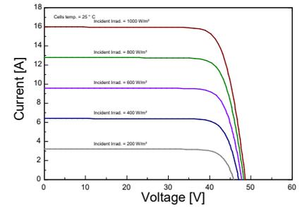
P-V CURVES OF PV MODULE (615W)
